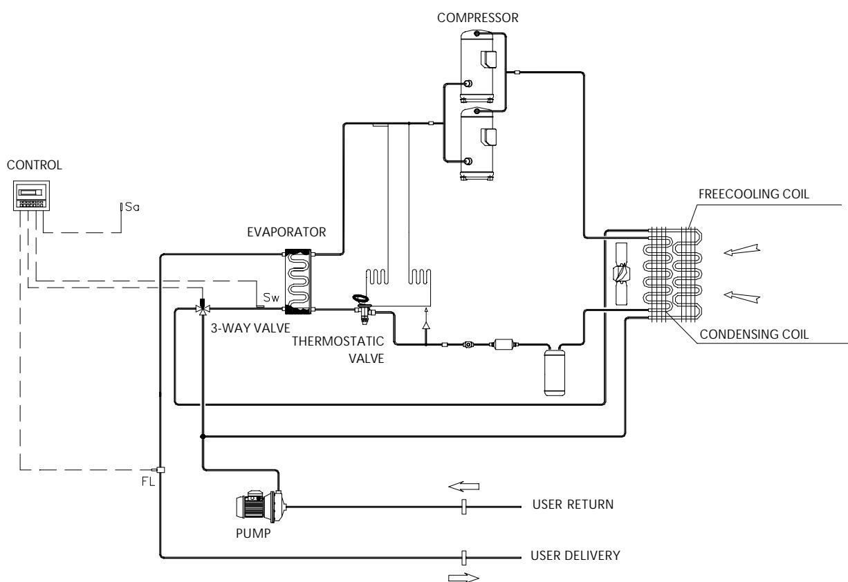
Another strong point of the Free Cooling range is the SCS (Split Coil System) control that guarantees control of condensation pressure also at low ambient air temperatures without influencing fan air flow, thereby enabling simultaneous operation of the free resource (ambient air) and that provided by the cooling cycle. This minimises the energy spent by the compression system, while guaranteeing the required load.
